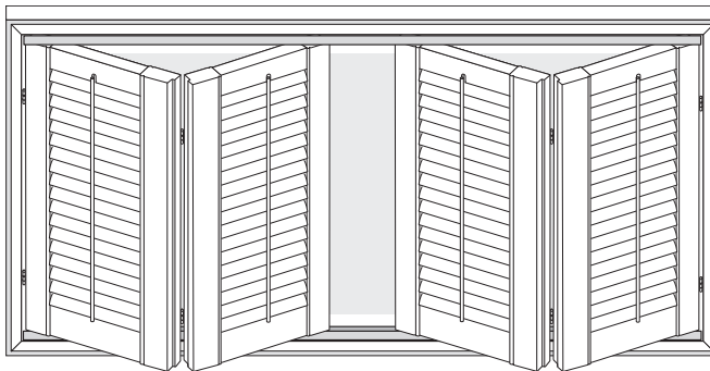
Bi-Fold Track System (wood only): Two or four panels are hinged together with a top and bottom track (see pages 47-49 for bi-fold information).
